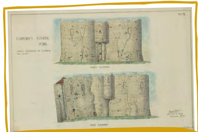
This architectural drawing made by the Office of Works in 1913 shows how the surviving shell of Clifford's Tower had seriously decayed by the 20th century.
