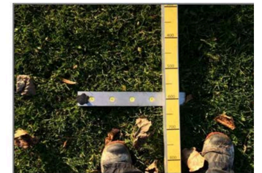
Plate 15: Minor undulation <5 mm
