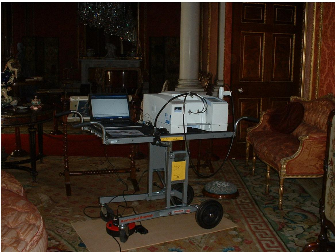
**Figure 12.4 – NIR spectrometer *in situ* at Brodsworth Hall**
