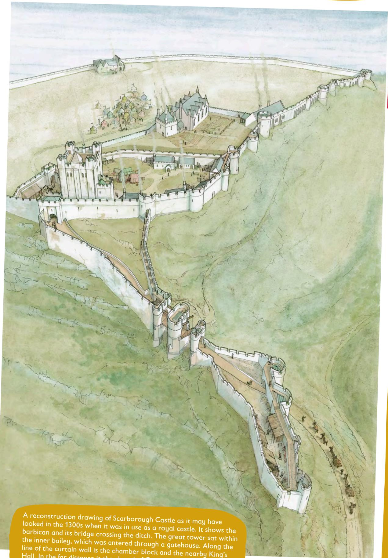
A reconstruction drawing of Scarborough Castle as it may have looked in the 1300s when it was in use as a royal castle. It shows the barbican and its bridge crossing the ditch. The great tower sat within the inner bailey, which was entered through a gatehouse. Along the line of the curtain wall is the chamber block and the nearby King's Hall. In the far distance is the chapel of Our Lady on the site of the former Roman signal station.
